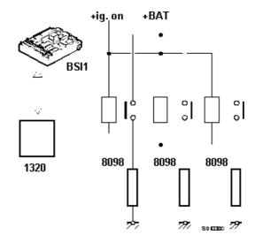
Assembly with 3 relays and 3 resistors
