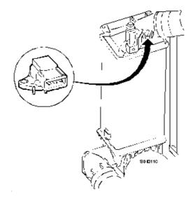
The inlet manifold pressure sensor is located on the outlet of the air/air heat exchanger.
