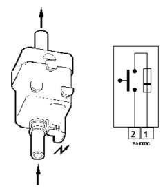
The fuel heater heats the fuel from the fuel tank.
