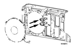
The 2 resistors are located on the front panel, near to the air/air exchanger and the fan unit.
