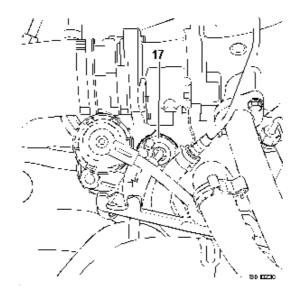
17 - inlet air heater throttle control electrovalve
